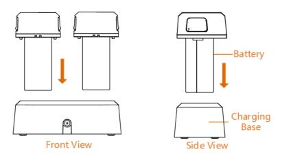
Figure 2-2 Charge Battery
